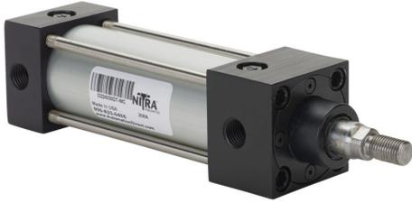
NITRA pneumatic cylinder, NFPA tie rod, 1-1/2in bore, 5/8in rod diameter, 3in stroke, double acting, magnetic piston, front and rear adjustable cushions, tapped end caps mount.
