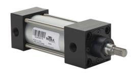
NITRA pneumatic cylinder, NFPA tie rod, 1-1/2in bore, 5/8in rod diameter, 2in stroke, double acting, magnetic piston, tapped end caps mount.
