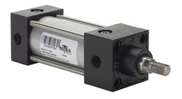
NITRA pneumatic cylinder, NFPA tie rod, 1-1/2in bore, 5/8in rod diameter, 2in stroke, double acting, magnetic piston, front and rear adjustable cushions, tapped end caps mount.
