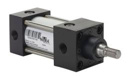
NITRA pneumatic cylinder, NFPA tie rod, 1-1/2in bore, 5/8in rod diameter, 1in stroke, double acting, magnetic piston, front and rear adjustable cushions, tapped end caps mount.
