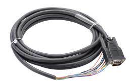
DirectLOGIC DL205 programming cable, 12ft cable length, shielded, 15-pin male HD15 to pigtail. For use with DL06, D2-250-1, D2-260 and D2-262 CPUs and D0-DCM communication module.
