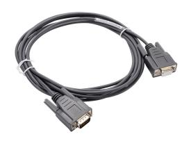
DirectLOGIC DL205 programming cable, 12ft cable length, shielded, 9-pin female D-sub to 15-pin male HD15. For use with DL06, D2-250-1, D2-260 and D2-262 CPUs and D0-DCM communication module.
