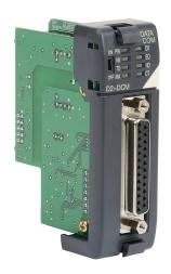
DirectLOGIC DL205 communication module, DirectNET and Modbus RTU, 1 port, (1) RS-232/RS-422 port(s). For use with DL205 PLCs.
