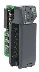
DirectLOGIC DL205 pulse combo module, 5 kHz maximum switching frequency, 4 high-speed input point(s), sinking/ sourcing, single-ended encoder input(s), 2 high-speed output point(s), sinking, single-ended output(s).
