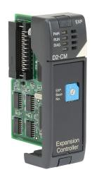
DirectLOGIC DL205 expansion unit, local expansion I/O. For use with D2-250-1, D2-260 or D2-262 CPUs.
