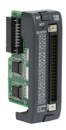
DirectLOGIC DL205 discrete output module, 32-point, 12-24 VDC, sinking, 4 isolated common(s), 8 point(s) per common, 0.1A/point, 3.2A/module. Requires ZIPLink pre-wired cable.
