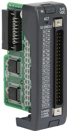
DirectLOGIC DL205 discrete input module, 32-point, 5-12 VDC, sinking/sourcing, 4 isolated common(s), 8 point(s) per common.
