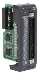
DirectLOGIC DL205 discrete input module, 32-point, 5-12 VDC, sinking/sourcing, 4 isolated common(s), 8 point(s) per common.
