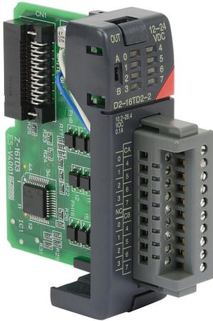
DirectLOGIC DL205 discrete output module, 16-point, 12-24 VDC, sourcing, 2 isolated common(s), 8 point(s) per common, 0.1A/point, 1.6A/module. Removable terminal block included.
