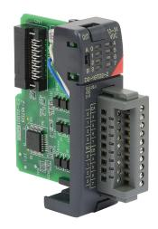
DirectLOGIC DL205 discrete output module, 16-point, 12-24 VDC, sourcing, 2 isolated common(s), 8 point(s) per common, 0.1A/point, 1.6A/module. Removable terminal block included.
