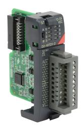
DirectLOGIC DL205 discrete output module, 16-point, 12-24 VDC, sinking, 1 common(s), 16 point(s) per common, 0.1A/point, 1.6A/module. Removable terminal block included.
