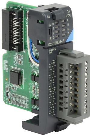
DirectLOGIC DL205 discrete input module, 16-point, 24 VDC, sinking/sourcing, 2 isolated common(s), 8 point(s) per common. Removable terminal block included.
