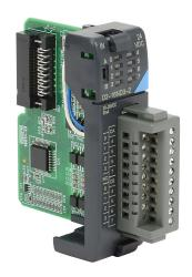
DirectLOGIC DL205 discrete input module, 16-point, 24 VDC, sinking/sourcing, 2 isolated common(s), 8 point(s) per common. Removable terminal block included.
