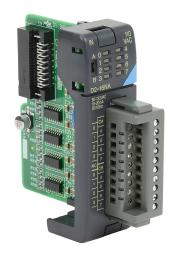
DirectLOGIC DL205 discrete input module, 16-point, 120 VAC, 2 isolated common(s), 8 point(s) per common. Removable terminal block included.
