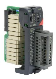
DirectLOGIC DL205 relay output module, 12-point, 6-24 VDC/6-240 VAC, (12) Form A, 2 common(s), 6 point(s) per common, 1.5A/point max, 3A/common. Removable terminal block included.
