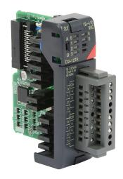
DirectLOGIC DL205 discrete output module, 12-point, 24-120 VAC, 2 isolated common(s), 6 point(s) per common, 0.3A/point, 1.8A/common. Removable terminal block included.
