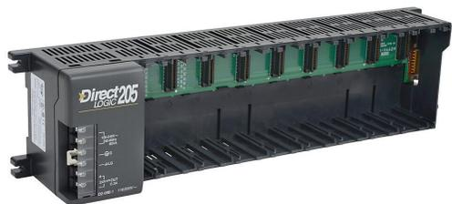
DirectLOGIC DL205 I/O base, 9-slot, DIN rail or panel mount, external 110-220 VAC required. 24 VDC 300 mA isolated auxiliary output power included.
