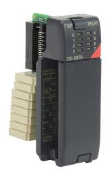
DirectLOGIC DL205 relay output module, 8-point, 6-24 VDC/6-240 VAC, (8) Form A, 1 common(s), 8 point(s) per common, 1A/point, 4A/module. Removable terminal block included.
