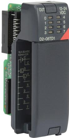
DirectLOGIC DL205 discrete output module, 8-point, 12-24 VDC, sinking, 1 common(s), 8 point(s) per common, 0.3A/point, 2.4A/module. Removable terminal block included.
