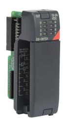
DirectLOGIC DL205 discrete output module, 8-point, 12-24 VDC, sinking, 1 common(s), 8 point(s) per common, 0.3A/point, 2.4A/module. Removable terminal block included.
