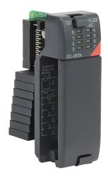
DirectLOGIC DL205 discrete output module, 8-point, 24-240 VAC, 1 common(s), 8 point(s) per common, 0.5A/point, 4A/common. Removable terminal block included.
