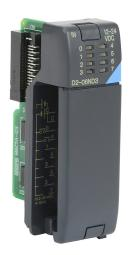
DirectLOGIC DL205 discrete input module, 8-point, 12-24 VDC, sinking/sourcing, 1 common(s), 8 point(s) per common. Removable terminal block included.
