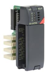
DirectLOGIC DL205 relay output module, 4-point, 6-24 VDC/6-240 VAC, (4) Form A, 4 isolated common(s), 4 point(s) per common, 4A/point, 8A/module. Removable terminal block included.
