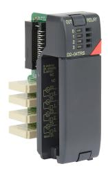
DirectLOGIC DL205 relay output module, 4-point, 6-24 VDC/6-240 VAC, (4) Form A, 4 isolated common(s), 4 point(s) per common, 4A/point, 8A/module. Removable terminal block included.
