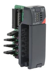
DirectLOGIC DL205 discrete output module, 4-point, 12-24 VDC, sinking, 1 common(s), 4 point(s) per common, 4A/point, 8A/module. Removable terminal block included.
