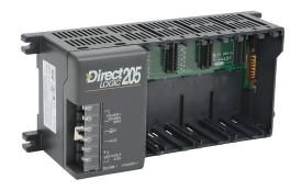
DirectLOGIC DL205 I/O base, 4-slot, DIN rail or panel mount, external 110-220 VAC required. 24 VDC 300 mA isolated auxiliary output power included.
