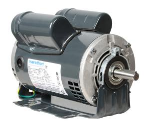
Marathon standard efficiency AC induction motor, fan and blower, 1-1/2hp, 1-phase, 115/208-230 VAC, 3600rpm, ODP, NEMA 56 frame, rolled steel, resilient base mount.
