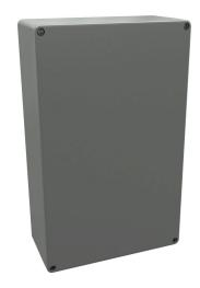
Stahlin DuraBoxx series enclosure, NEMA 1/3/3S/4X/6/6P/12, 400 x 250 x 121mm (HxWxD), fiberglass reinforced polyester, Pantone 428 C glacier gray, screw cover.
