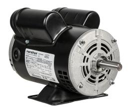
Marathon standard efficiency AC induction motor, pressure washer definite purpose, 1hp, 1-phase, 115/208-230 VAC, 3600rpm, ODP, 56 frame, rolled steel, rigid base mount.
