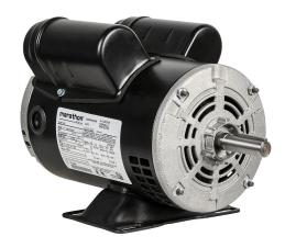
Marathon standard efficiency AC induction motor, pressure washer definite purpose, 1hp, 1-phase, 115/208-230 VAC, 3600rpm, ODP, NEMA 56 frame, rolled steel, rigid base mount.
