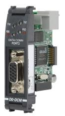
DirectLOGIC DL05/06 communication module, DirectNET and Modbus RTU, 2 ports, (1) RS-232 (RJ12) and (1) RS-232/RS-422/ RS-485 (HD15) port(s). For use with DL05 and DL06 PLCs.
