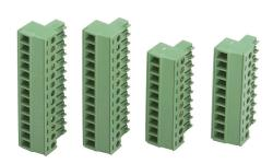
DirectLOGIC DL05/06 terminal block kit, 90-degree screw type, replacement. For use with DL05/06 I/O modules. Includes (2) 10-pin 3.5mm terminal blocks and (2) 13-pin 3.5mm terminal blocks.
