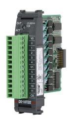
DirectLOGIC DL05/06 discrete output module, 10-point, 12-24 VDC, sourcing, 2 common(s), 5 point(s) per common, 0.3A/point, 1.5A/common. Removable terminal block included.
