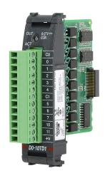
DirectLOGIC DL05/06 discrete output module, 10-point, 6-24 VDC, sinking, 2 common(s), 5 point(s) per common, 0.3A/point, 1.5A/common. Removable terminal block included.
