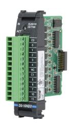
DirectLOGIC DL05/06 discrete input module, 10-point, 12-24 VDC, sinking/sourcing, 2 isolated common(s), 5 point(s) per common. Removable terminal block included.
