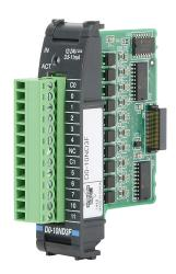
DirectLOGIC DL05/06 discrete input module, 10-point, 12-24 VDC, sinking/sourcing, fast response, 2 isolated common(s), 5 point(s) per common. Removable terminal block included.
