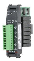
DirectLOGIC DL05/06 relay output module, 8-point, 6-24 VDC/6-240 VAC, (8) Form A, 2 isolated common(s), 4 point(s) per common, 1A/point, 4A/common. Removable terminal block included.
