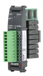
DirectLOGIC DL05/06 relay output module, 8-point, 6-24 VDC/6-240 VAC, (8) Form A, 2 isolated common(s), 4 point(s) per common, 1A/point, 4A/common. Removable terminal block included.
