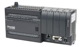
DirectLOGIC DL06 PLC, 12-24 VDC required, serial ports, Discrete Input: 20-point, DC, Discrete Output: 16-point, relay.
