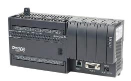
DirectLOGIC DL06 PLC, 12-24 VDC required, serial ports, Discrete Input: 20-point, DC, Discrete Output: 16-point, sourcing.
