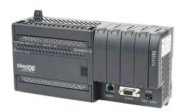
DirectLOGIC DL06 PLC, 12-24 VDC required, serial ports, Discrete Input: 20-point, DC, Discrete Output: 16-point, sinking.
