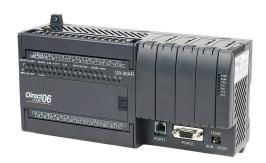
DirectLOGIC DL06 PLC, 120-240 VAC required, serial ports, Discrete Input: 20-point, AC, Discrete Output: 16-point, relay.
