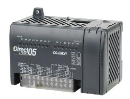
DirectLOGIC DL05 PLC, 120-240 VAC required, serial ports, Discrete Input: 8-point, DC, Discrete Output: 6-point, relay.
