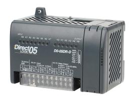
DirectLOGIC DL05 PLC, 12-24 VDC required, serial ports, Discrete Input: 8-point, DC, Discrete Output: 6-point, relay.
