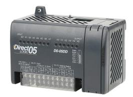
DirectLOGIC DL05 PLC, 120-240 VAC required, serial ports, Discrete Input: 8-point, DC, Discrete Output: 6-point, sinking.
