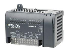
DirectLOGIC DL05 PLC, 120-240 VAC required, serial ports, Discrete Input: 8-point, AC, Discrete Output: 6-point, relay.
