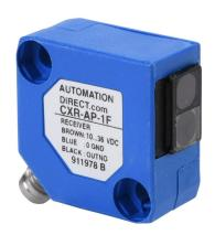
AutomationDirect photoelectric sensor, rectangular, plastic housing, through-beam receiver, 6m sensing distance, 10-36 VDC operating voltage, dark-on, PNP, 3-wire, 3-pin M8 quick-disconnect.
