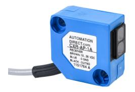
AutomationDirect photoelectric sensor, rectangular, plastic housing, through-beam receiver, 6m sensing distance, 10-36 VDC operating voltage, dark-on, PNP, 3-wire, pigtail.
