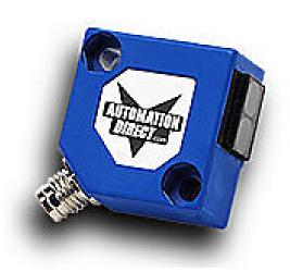
AutomationDirect photoelectric sensor, rectangular, polarized retroreflective, visible red light emission, 2m sensing distance, dark-on, PNP, potentiometer, 3-wire, 3-pin M8 quick-disconnect.
