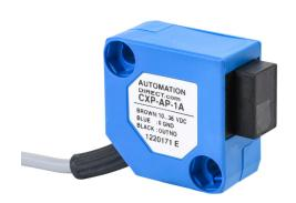
AutomationDirect photoelectric sensor, rectangular, polarized retroreflective, visible red, 2m sensing distance, dark-on, PNP, potentiometer, 3-wire, pigtail.
