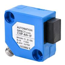
AutomationDirect photoelectric sensor, rectangular, polarized retroreflective, visible red, 2m sensing distance, dark-on, NPN, potentiometer, 3-wire, 3-pin M8 quick-disconnect.
