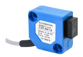
AutomationDirect photoelectric sensor, rectangular, polarized retroreflective, visible red light emission, 2m sensing distance, dark-on, NPN, potentiometer, 3-wire, pigtail.
