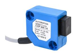
AutomationDirect photoelectric sensor, rectangular, polarized retroreflective, visible red, 2m sensing distance, dark-on, NPN, potentiometer, 3-wire, pigtail.
