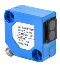
AutomationDirect photoelectric sensor, rectangular, plastic housing, through-beam emitter, infrared light emission, 6m sensing distance, 10-36 VDC operating voltage, 3-wire, 3-pin M8 quick-disconnect.
